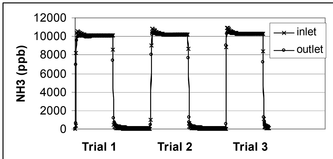
Figure 8. Adsorption – desorption curves of \text{NH}_3 on 46 m Teflon Tubing at concentrations of 10 ppm.
