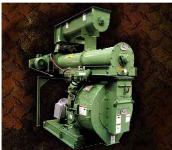
Figure 1. The California Pellet Mill Model 7000 (CPM 7000) used to pellet cotton gin trash.
