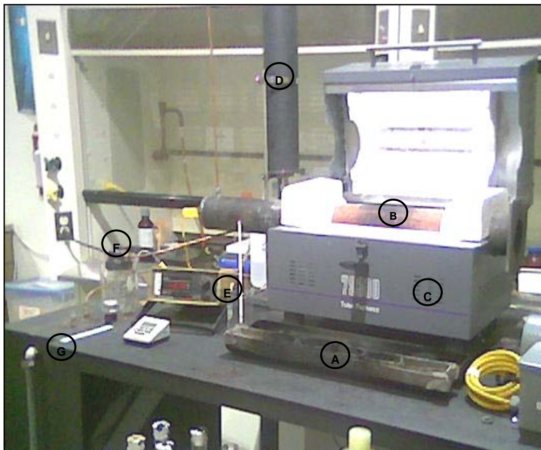
Figure 1. The pyrolysis set-up used in the experiment showing the following parts: (A) steel tray, (B) horizontal tube reactor, (C) tube furnace, (D) condenser, (E) thermocouple reader, (F) cold trap, and (G) displacement tanks.
