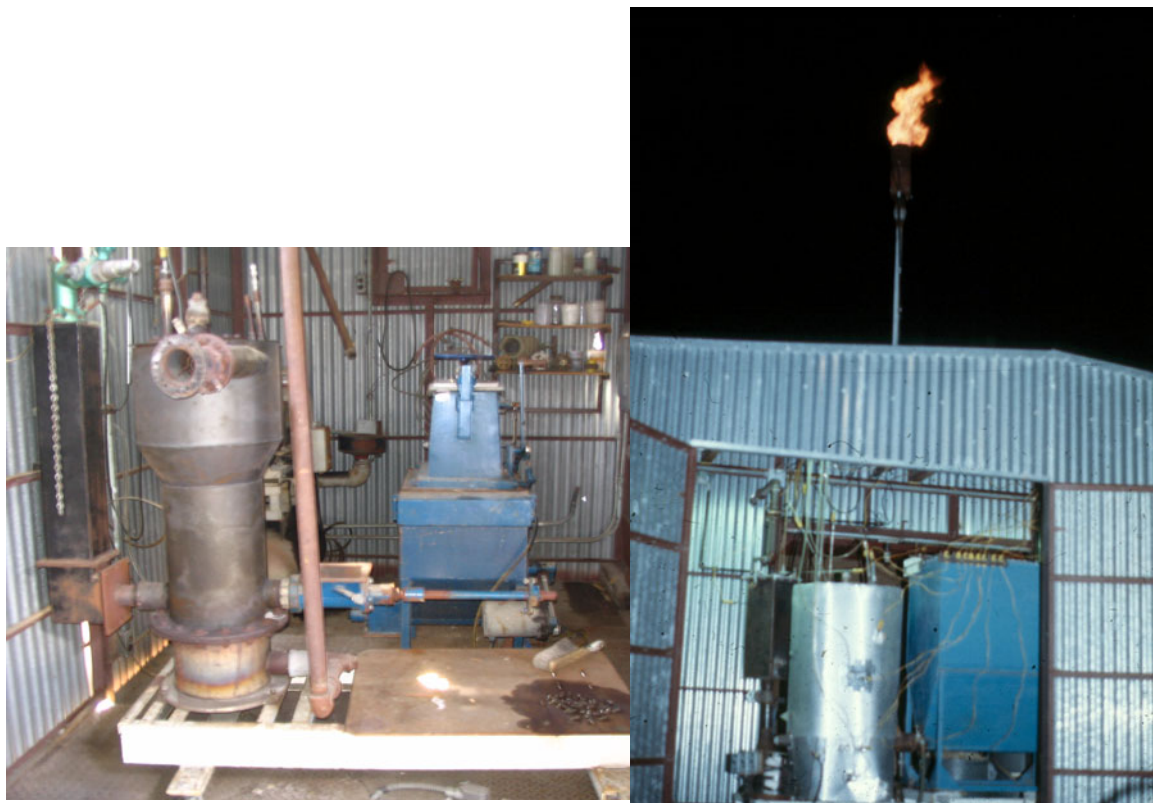
Figure 4. The pilot scale fluidized bed gasifier at TAMU.
